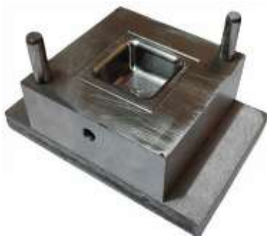
Fig. 7. Bottom die with plate
