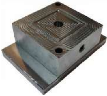
Fig. 6. Top die with plate
